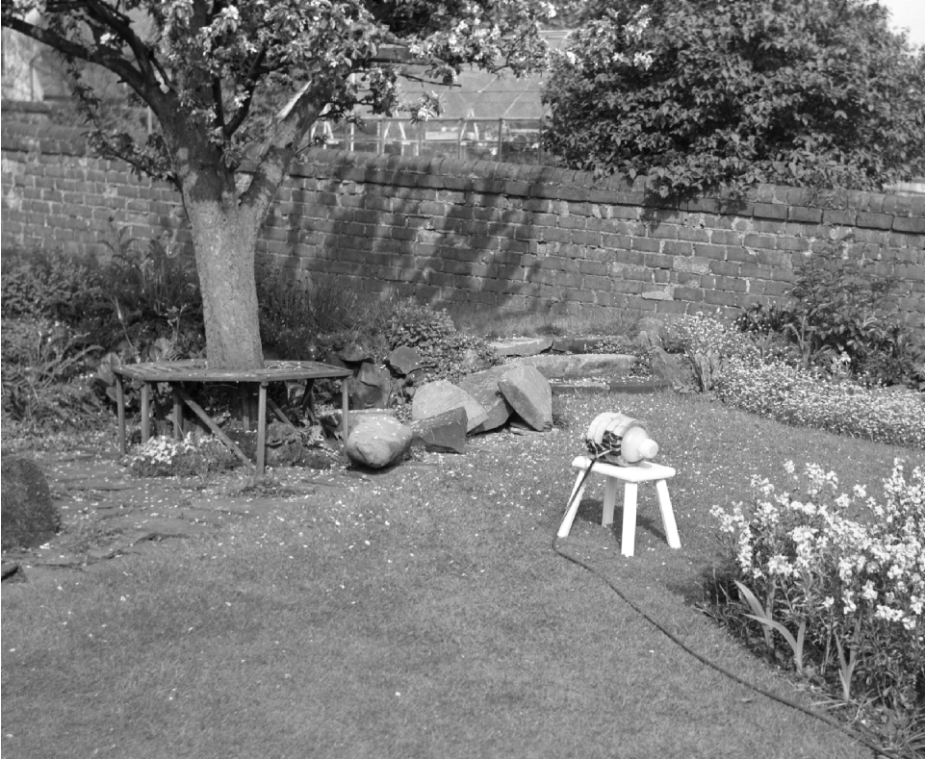
Fig. 3. Photograph of coil and sample bottle on a wooden iron-free stool during early tests in a countryside garden location
