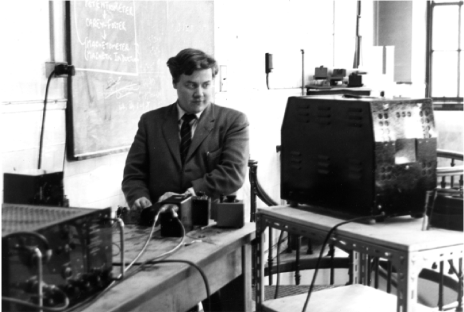
Fig. 6. A photograph taken during development and testing of the electronics and switching system in one of the Honours Natural Philosophy laboratories. A modified low noise nuclear physics amplifier and preamplifier used are on the left and an oscilloscope with a long persistence phosphor on the right. The sample coil was suspended outside the building for these tests
